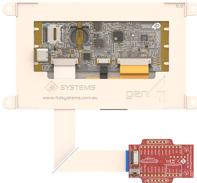
The 4D-UPA is connected to the ESP32 module using the supplied 30-way FFC Cable. The connectors on both the ESP32 module, and the 4D-UPA, are Top-Contact, meaning the FFC cable pins should be facing upwards, and the blue stiffener, should be facing down towards the PCB.
