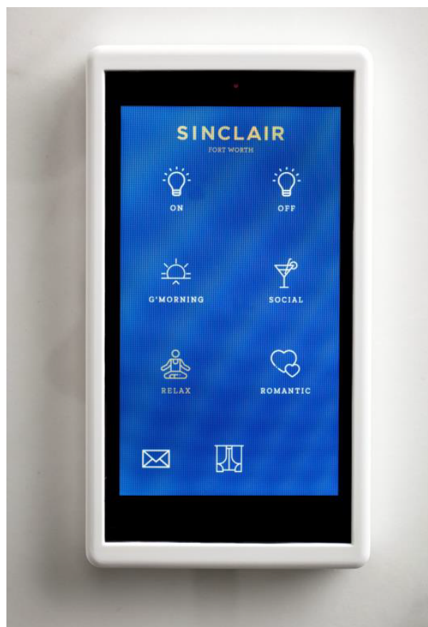
The Sinclair In-Room control interface, created using 4D SYSTEMS' 4Discovery-50
