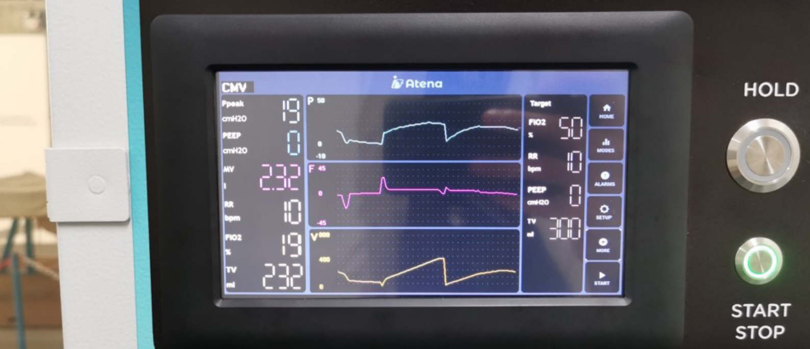
A close-up of the graphic user interface on The Atena, utilizing the gen4-uLCD-70DT
