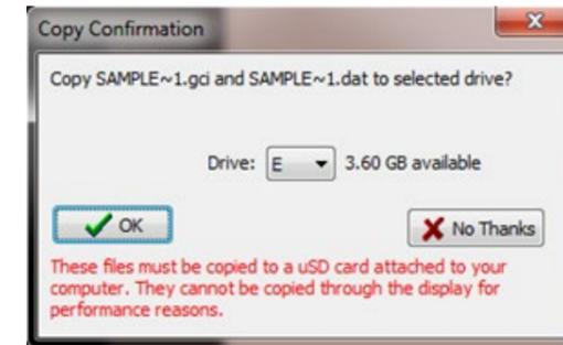
Click OK after the files are transferred to the microSD card. Unmount the microSD Card from the PC and insert it to the display module's microSD Card slot.
