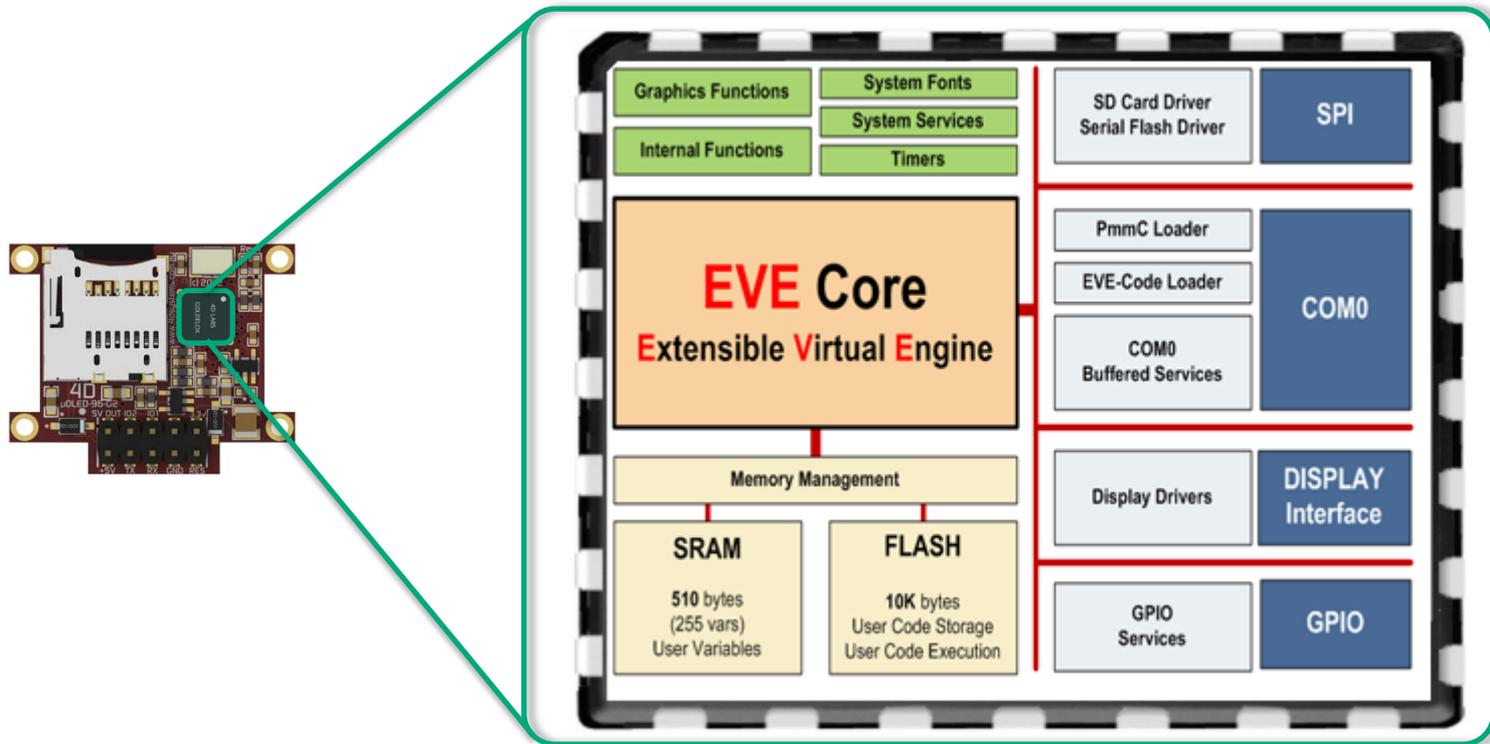
The GOLDELOX offers a complete suite of features, crafted to be at the forefront of any product requiring colour, animation, images and sound. The GOLDELOX is also powerful enough to control and communicate with peripheral devices over SPI, One Wire or Serial Port.
