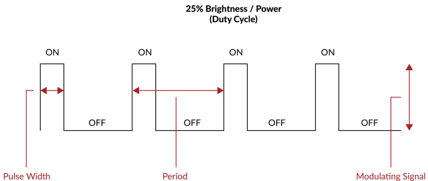
The screen's brightness is adjusted using PWM (Pulse Width Modulation)
