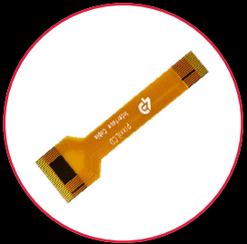
15-way to 30-way Flat Flex Cable (FFC)
